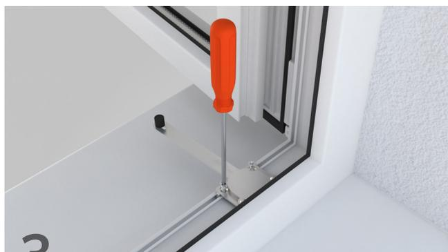
**3** Tighten the screws partially.
