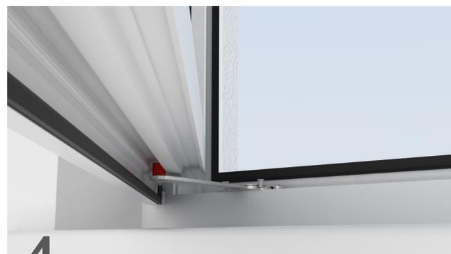
**4** Insert the Blockade arm into the groove window sash or balcony door groove.
